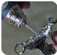
打磨支架缝隙 For Trimming Metal
