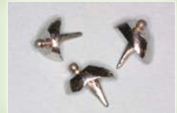
Cast post and sphere. It is also possible to place the sphere off center in respect to the long axis of the post.
