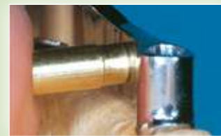
Insert the housing shaper into the hole and lock it in place using resin. Be sure not to go past the "STOP" when applying resin.
