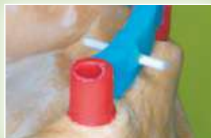
Insert the ceramic pin through the hole.
