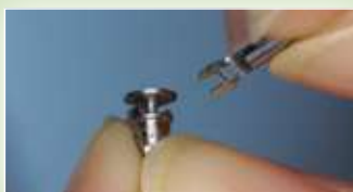
Insert the locking key into the pre-fabricated housing guide. The "key-ring" mechanism is now locked.
